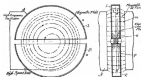
Fig:7.1. Diagram of cyclotron operation from Lawrence's 1934 patent
